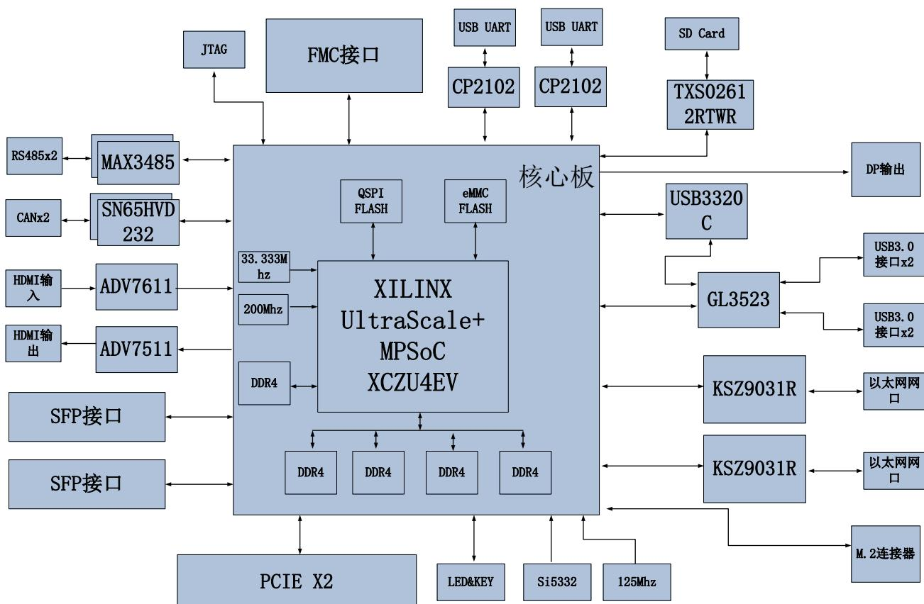
Figure 1-1-1: The Schematic Diagram of the AXU4EV-P
