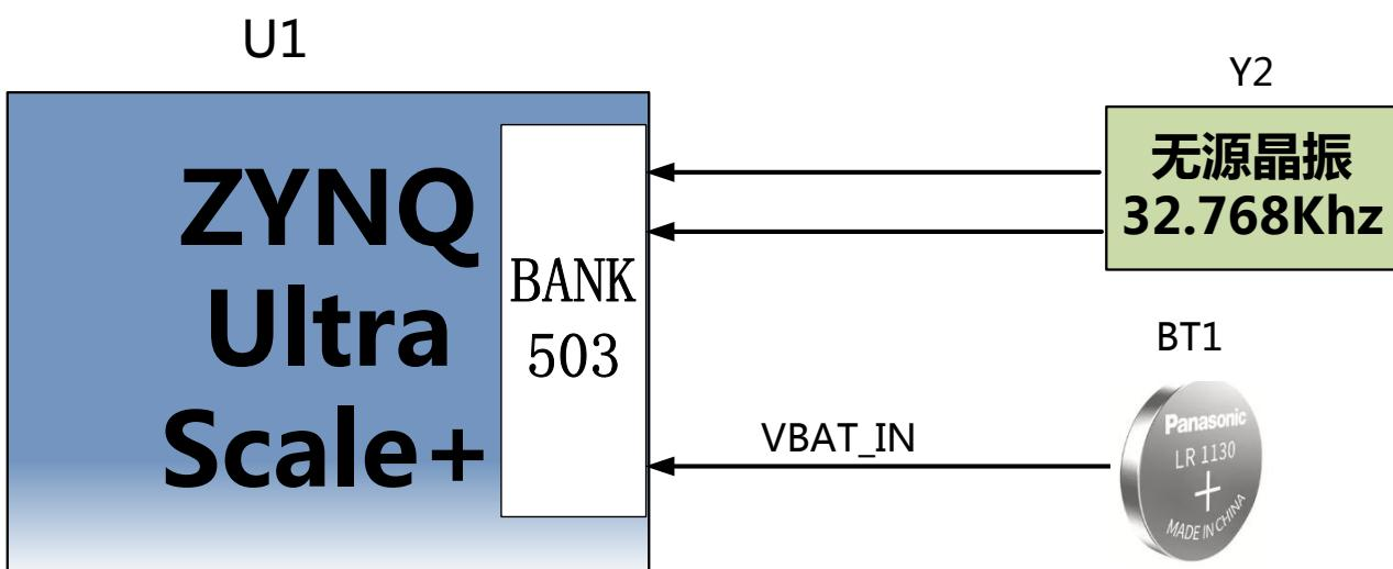
Figure 3-17-1: RTC Schematic
