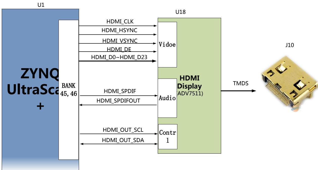
Figure 3-8-1: HDMI Output Interface Schematic
