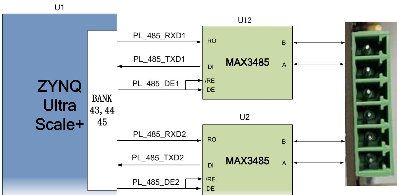
Figure 3-13-1: 485 Communication on the PL Side
