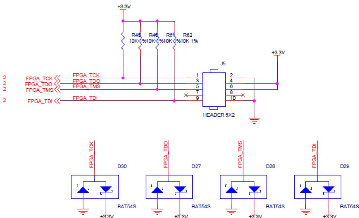
Figure 3-16-1: JTAG Interface Schematic
