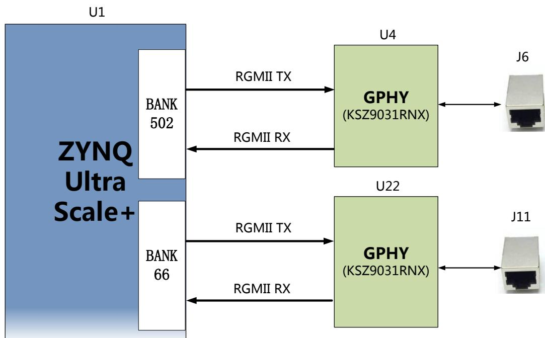
Figure 3-5-1: ZYNQ PS system and GPHY connection diagram
