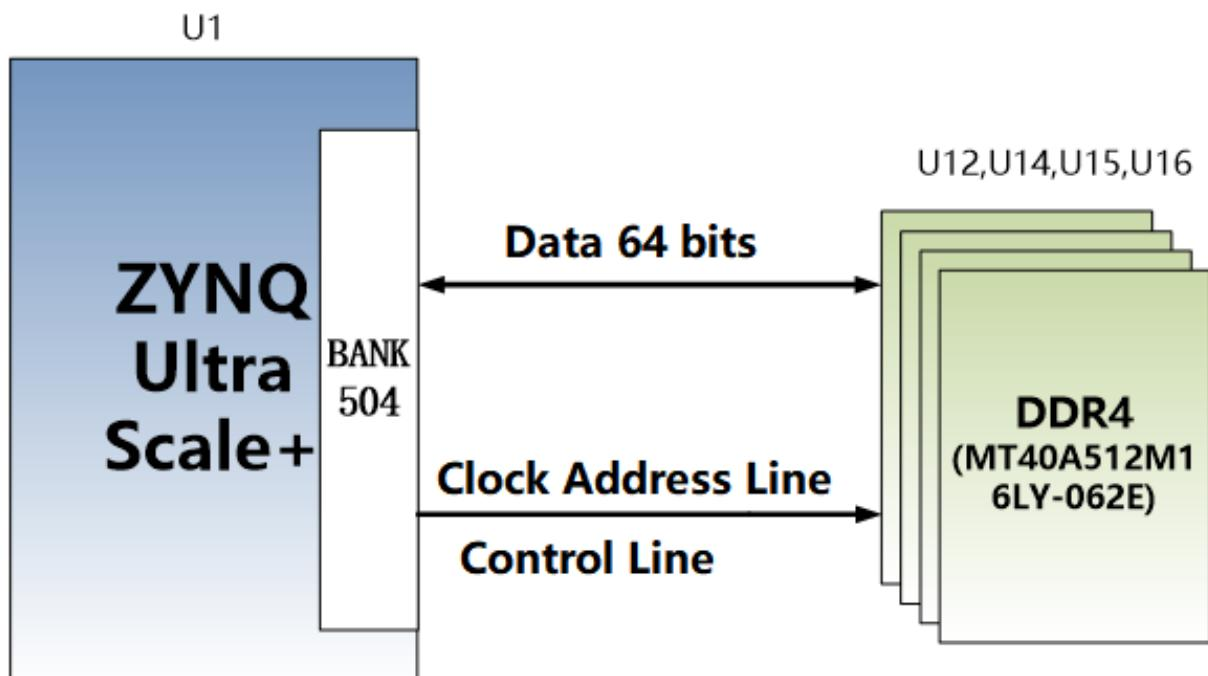
Figure 2-3-1: DDR3 DRAM schematic diagram
