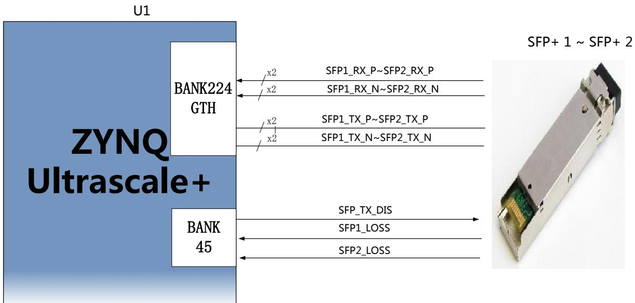
Figure 3-10-1: SFP Schematic
