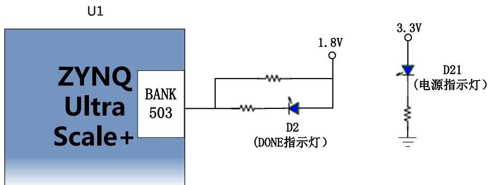
Figure 2-7-1: LED Schematic in the Core Board
