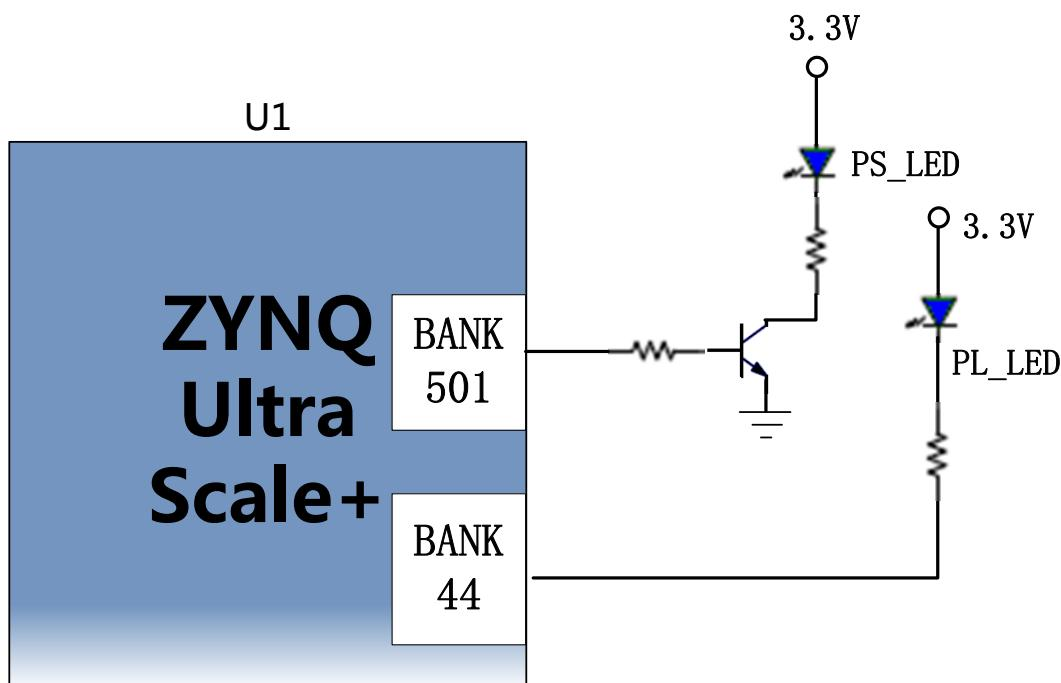
Figure 3-19-1: The User LEDs Hardware Connection Diagram
